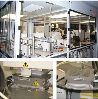
Figure 7. Photographs of linear track robotic system used for automated siRNA screening. Included in the system are 3 CyBi Well pipetting stations and 1 CyBi Disk pipetting station. The pictures below depict the easy installation and set up of the TipCharger system on the CyBi Disk.
